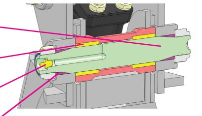
This system allows an easy elimination of play between pin and bushing caused by wear by tightening the nuts of the pin.
